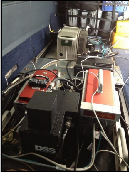
Furthest aft: Riegl VQ-820-G topo bathy lidar. Foreground: Applanix DSS DualCam digital aerial camera
